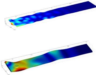
**Figure 4.** Simulation results of the plate to evaluate temperature rise in a crack at different excitation amplitudes.
