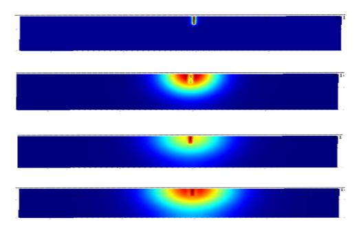
Figure 6. Numerical results of heat generation in plate with a crack, at different time steps. Heating is due to friction effect.
